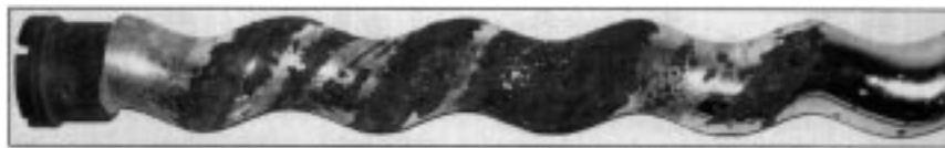
Figure 4. Failure of chrome plating due to corrosion of rotor base material (carbon steel)
